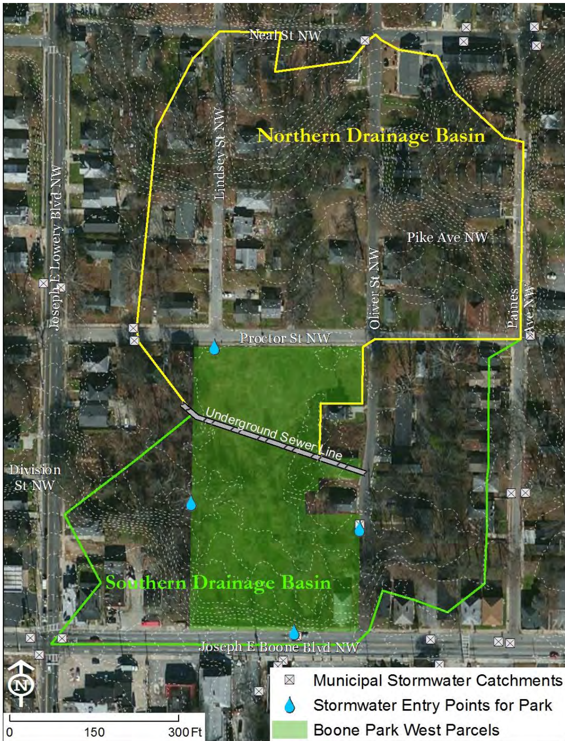
This figure illustrates the different drainage basins surrounding the park as well as the location of the large combined sewer trunk line that runs underneath the site.
